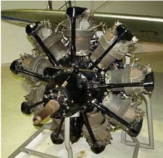
Bristol Mercury engine, first run 1925. 9 cylinder, air cooled single row piston radial engine.
